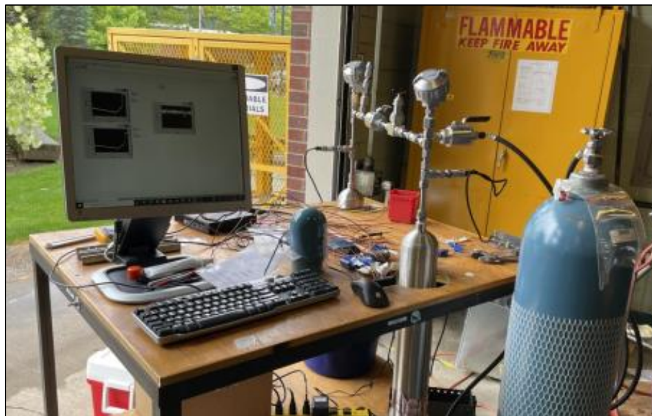
Figure 1: Laboratory Setup of Cold Storage Battery Test
