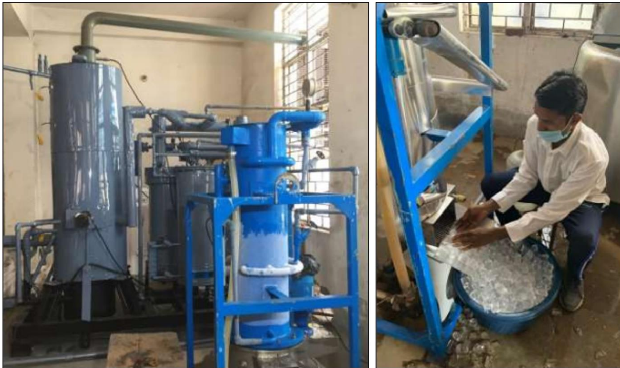
Figure 1: GreenCHILL™ Unit with Ice Maker (in Blue), and Producing Ice
